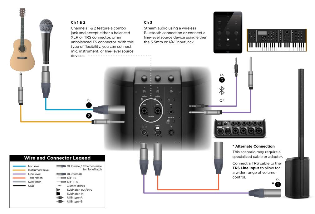
The L1 Pro8 isn't just for singer-songwriters and DJs; presenters need to be heard too. In this example, the wireless mic receiver can be connected to input 1 or 2. A PC laptop for multimedia presentations can connect to channel 3 either using a Bluetooth connection or the 3.5mm aux input. Level adjustments can either be made directly on the built-in mixer or from the L1 Mix app on a mobile phone or tablet.
